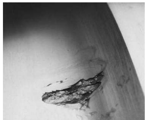
Fig. 5.2 Photo-illustration of fatigue damage on the raceway
