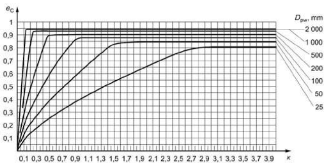
Fig. 5.7 Fouling factor for a circulating oil lubrication system with on-line filtration \beta_c = 200
